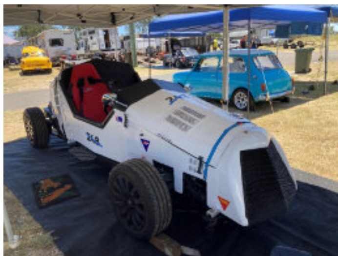
Above: Soft Serve from a three-quarter frontal view and Liam's handy work is well illustrated right down to a mesh grill, foot step, battery isolator switch and caravan style bonnet catches. Source: John Carson
